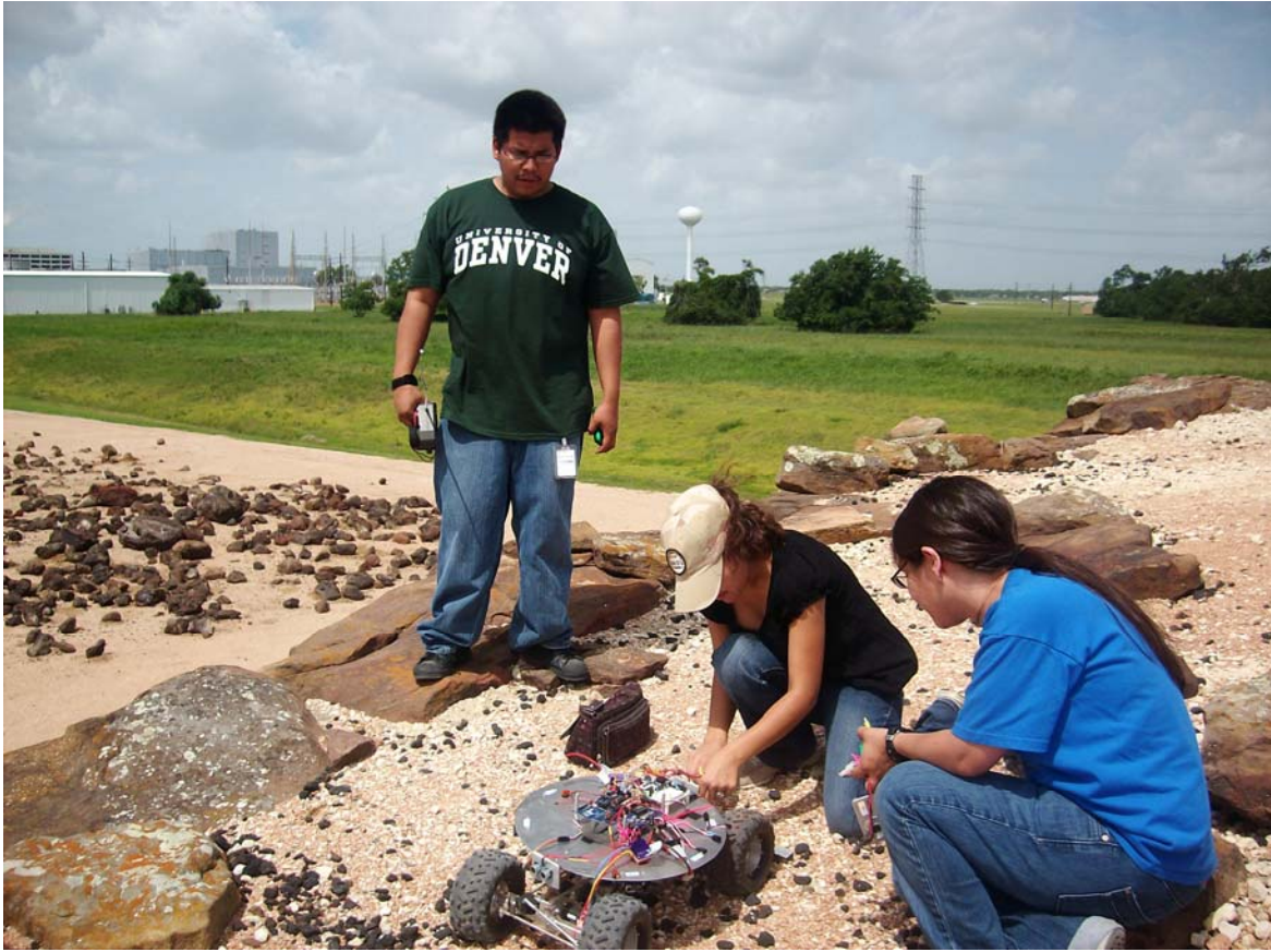
SIPI team members are testing their Rock crawler rover platform on the NASA JSC Rock Yard.
